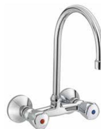
RAK35001SU Dual controlled wall mounted sink mixer DN 15 swivel U spout aerator M22 x 1 flow class A S- unions 1/2 inch x 3/4 inch European standard- EN200
