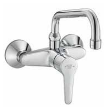
RAK10028 Wall mounted single lever sink mixer DN 15 ceramic cartridge-K35 swivelling (185°) spout l = 200 mm aerator M 22 x 1 flow class A S- unions 1/2 X 3/4 inch European standard - EN 817
