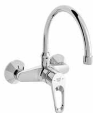
RAK30029SU Wall mounted single lever sink mixer DN 15 ceramic cartridge-K35 swivelling (185°) U spout l =210 mm aerator M 22 x 1 flow class A S- unions 1/2 X 3/4 inch European standard- EN 817
