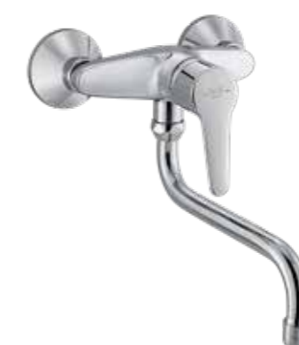
RAK10008 Wall mounted single lever sink mixer DN 15 ceramic cartridge-K35 swivelling (185°) spout l = 200 mm aerator M 22 x 1 flow class A S- unions 1/2 X 3/4 inch European standard- EN 817
