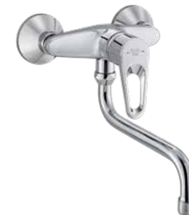
RAK30008 Wall mounted single lever sink mixer DN 15 ceramic cartridge-K35 swivelling (185°) spout l = 200 mm aerator M 22 x 1 flow class A S- unions 1/2 X 3/4 inch European standard- EN 817
